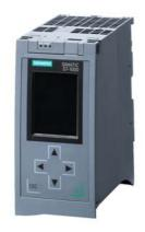
\*\*\*Spare part\*\*\* SIMATIC S7-1500, CPU 1516-3 PN/DP, Central processing unit with Work memory 1 MB for program and 5 MB for data, 1st interface, PROFINET IRT with 2-port switch, 2nd interface, Ethernet, 3rd interface, PROFIBUS, 10 ns bit performance, SIMATIC Memory Card required
